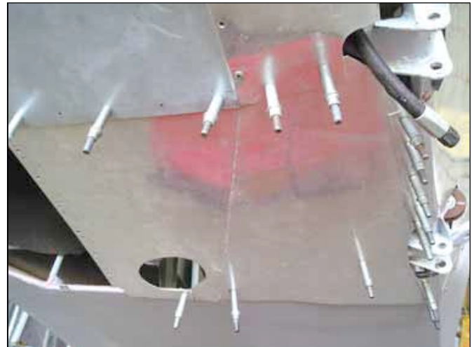
To keep the sheet metal around the struts from being a cut and try operation, do it first in poster board. Leave room for the struts to flex and for clearance around the filler plug. To accurately locate the hole in the aluminum, a) make a poster-board pattern for the entire piece b) make a separate hand-sized pattern with just the hole in it, c) With the struts attached, slide the small pattern around the strut, slide it up to the main pattern, which has a large hole in it, and tape it in place. This gives a perfectly placed hole in the pattern.
