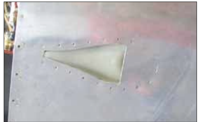
NACA scoops are available from a variety of aircraft supply houses. Although the concept is good, they have to be properly located to work well but they are the most low drag way of getting air into the ventilation system. This one is mounted in the boot cowl and feeds eyeball vents under the panel.
