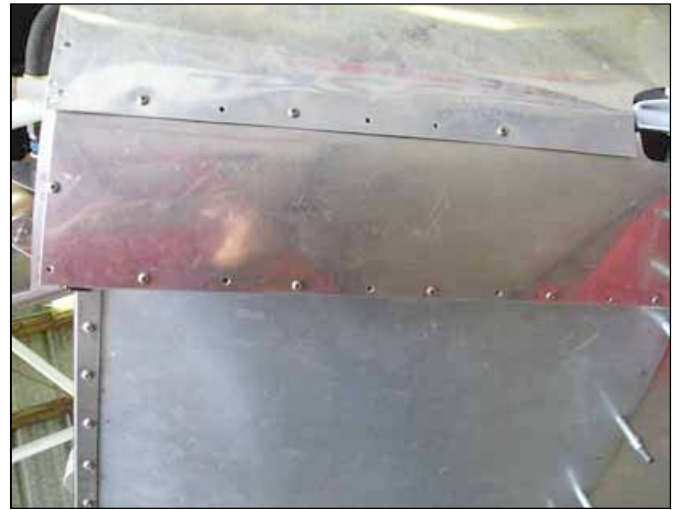
Lower left view of the boot cowl, looking up, nose to left. The lower corners of the cowl are to be removable for inspections. Put nutplates on the edges of the removeable panel.
