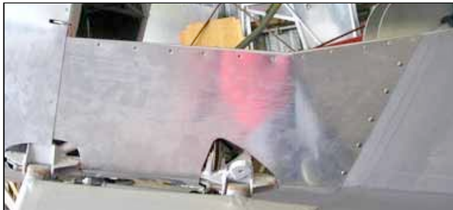
The piece of aluminum that goes under the doors is provided, but is optional. The prototypes didn't have it and it doesn't show in the plans. However, it provides a convenient place to securely fasten the wing root and landing gear fairings and cleans up the transition to the bottom sheet metal.
