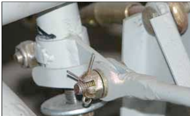
This is the way the seat latch looks from the front, when assembled. The short "T" handle goes under the right seat to clear to the flap handle. Drill holes in the track on 1" intervals.
