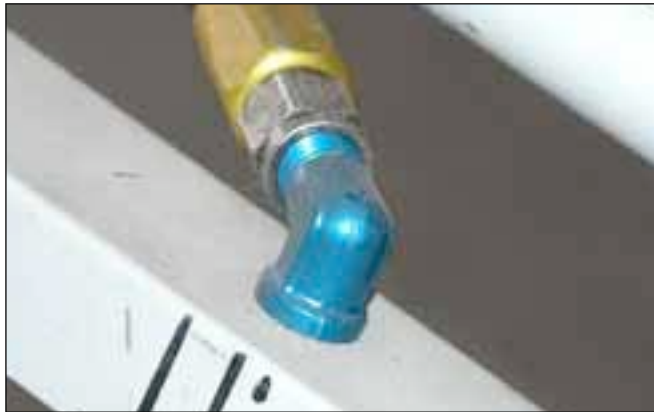
Connect a flex line to a bulkhead fitting at the top of the gear leg. where it goes into the fuselage.
