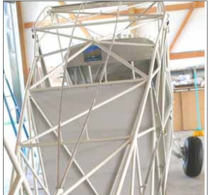
The stringers on both the sides and the top should form a pleasing line, when viewed from the rear. .
