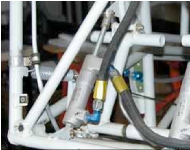
This is the Gerdes Long Shaft master cylinder for use with a firewall mounted reservoir, If a short shaft cylinder is used, a clevis fork can make up the difference in length. All of the pivot bolts need to be drilled/pinned bolts or clevis pins. The rule is that anything that rotates needs a cotter pin.
