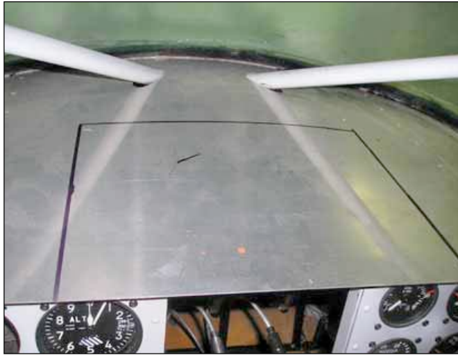
The access cover on the top of the panel should be cut after the sheet metal in the area is completely installed. Make a cover that laps on the outside edges of the hole and rivet a piece to the leading edge of that cover to form a lip that goes under the panel top and holds the cover in place.
