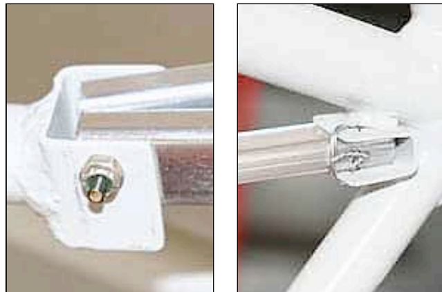
When attaching the stringers you'll find some odd areas, such as at the front of the vertical fin (left) where you'll have to pad it to give the fabric a smooth contact area. Doubled safety wire can be used to attach in some cases (right).
