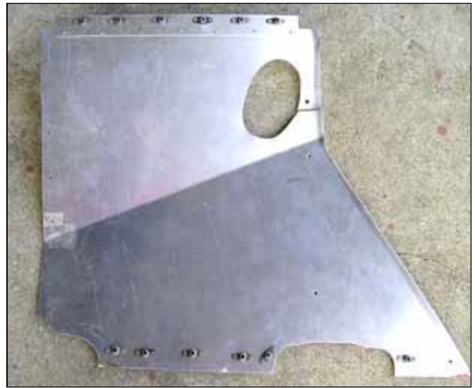
The bottom panel that goes from the landing gear shock strut to the side of the fuselage. The top hole is for the shock strut, the bottom left for the landing gear fitting the the lower right cut for the rear landing gear fitting and lift strut. The break in the surface is not as severe as it appears. It is a slight crease to line up with the belly stringers.
