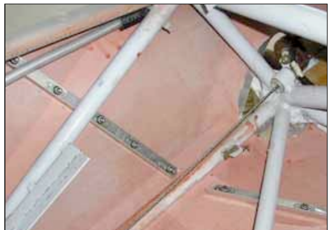
An attaching angle must be Adel clamped to the tubing to provide a place for the fabric to terminate and a place to attach the rear belly metal. Use hardware store aluminum angle.
