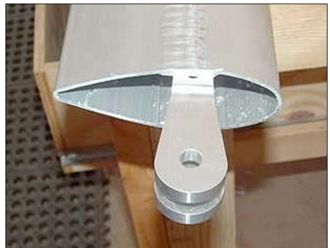
When the strut is squeezed to dimension, the fittings should barely slide inside with a minimum of tapping.
