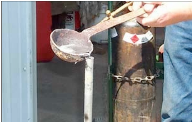
The tube can be clamped against something or stuck in the ground. Warm it before pouring the lead in.
