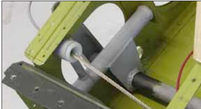
Sand the paint off the inside of the pivot bushing and the tube and it'll be easier to insert it and it will work much easier.
