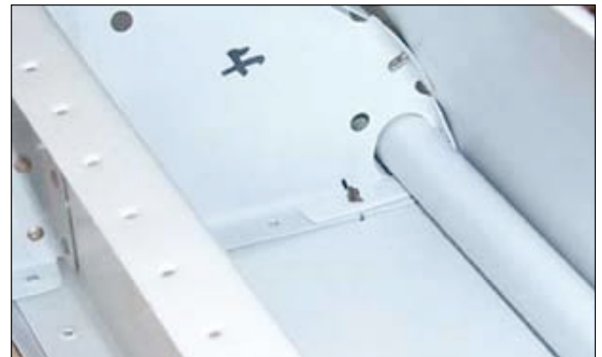
Inside forward view of an aileron nose: note the balance tube at the very forward part of the aileron. This area is closed up on kit ailerons so you can't see the tube.
