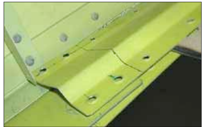
A few wings were produced in which the stiffener was too long and it interferes with the root rib. Trim off about 3/4" with a Dremel tool being careful not to cut the skin. Protect it with scrap aluminum.
