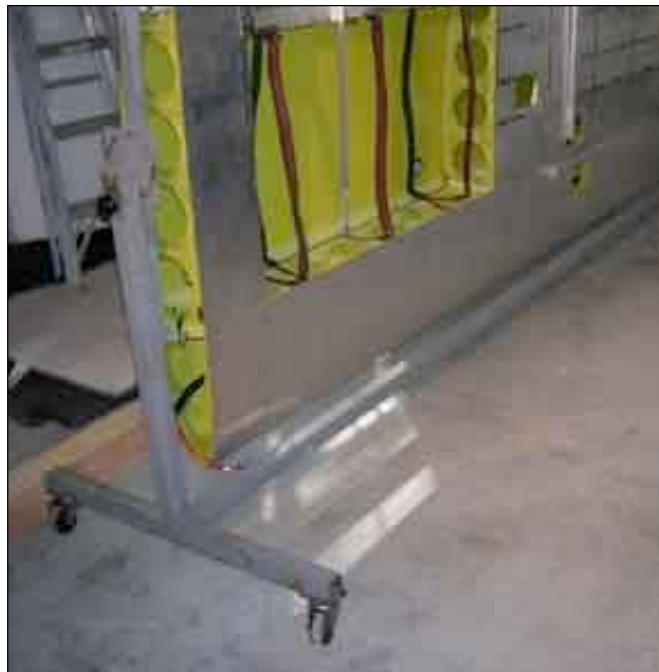
The wings don't weigh very much (150 pounds), but they are not only awkward but very easily damaged. Plus, you're always wishing you could get at the other side.
