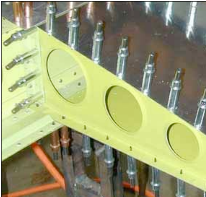
Left wing root. Notice how the bottom skin stiffener abuts the flange. You'll use the plywood template for aligning the ribs with
