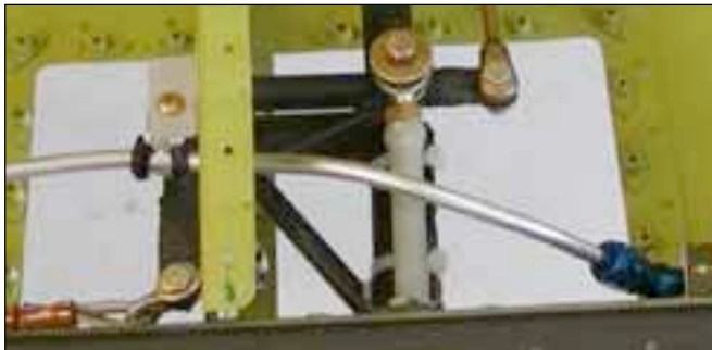
Aileron bellcrank. Here you can clearly see the cable at the bottom of the picture that is connected to the other wing. At the lower right you can see the fuel pump and the transfer line.
