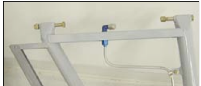
Install a 90-degree bulkhead fitting at the top of the gear leg and a flex-line from there to the brake line inside the fuselage. This is to allow the gear leg to move.
