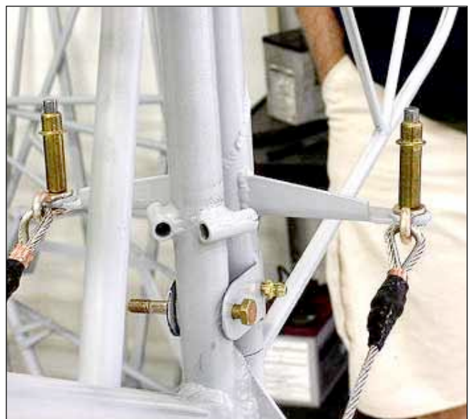
The rudder horn. Note the shackles and Nicopressed cables.
