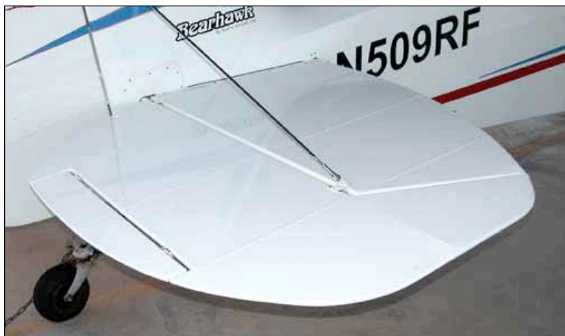
The tail is inserted in fittings and in a short carry-through tube at the front. All holes were drilled with the tail installed on your airplane so, if the holes don't line up, you have it together wrong. The early, big trim tab is shown.
