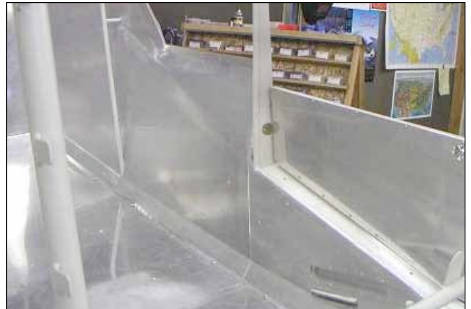
Another view of the cable covers down the walls.
