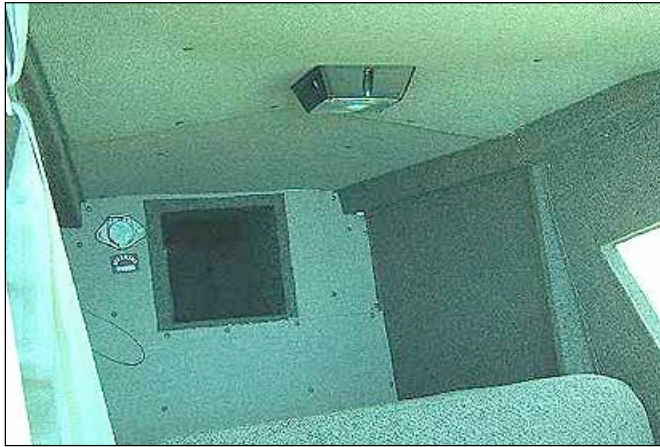
This builder went for a square ski tube that goes back several feet. He also installed a ground power plug in the upper left corner.
