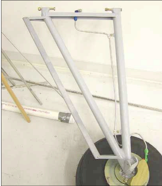
Typical brake line routing, although it is advisable to have the last part of the line going into the caliper be a flexible line. Matco brakes are shown.
