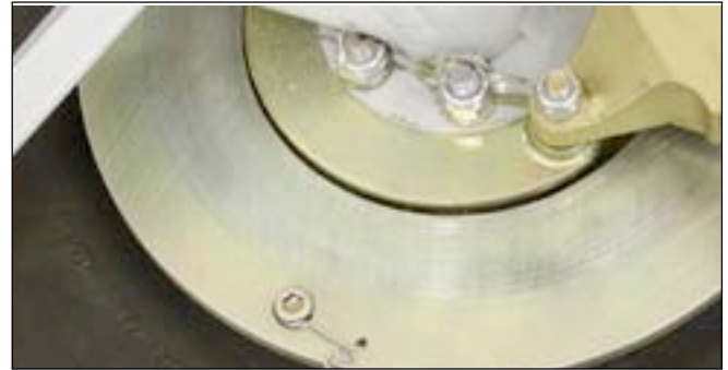
The clearance for the caliper nuts is minimal and may require grinding at least one nut for clearance. Three 5/16" bolts is adequate for the installation.
