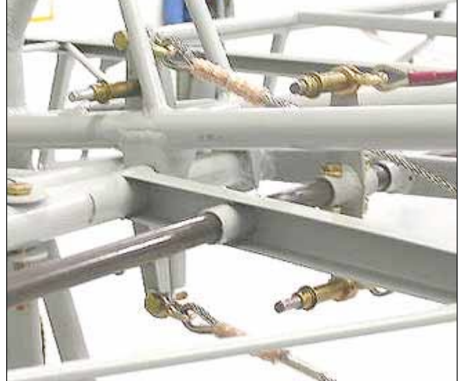
The relationship of the elevator horns and the trim horns are clearly seen with the trim horns being on the black tube.
