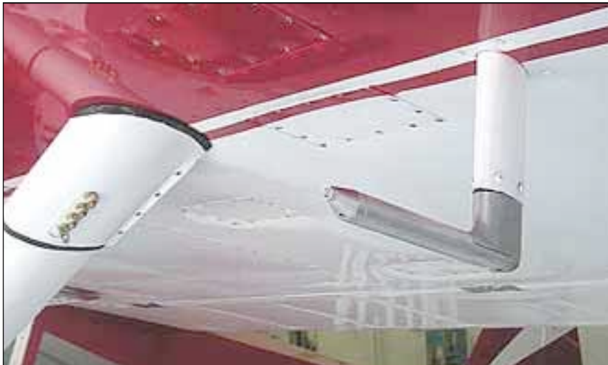
One of the more common pitot systems, the AN5812, comes in a heated version and depends on ports on both sides of the fuselage for static pressure .
