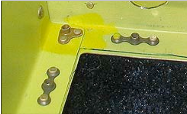
The K1000 nutplates install easily. If the corner hole is moved in a little from this position, a regular nutplate can bridge it. Otherwise, use the MS21073-06 as shown. Note the nice radius in the corner of the cut-out. This prevents stress cracks.
