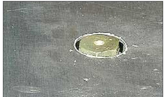
A flush mount (Wicks CAV 110) quick drain is recommended for all the tanks..
