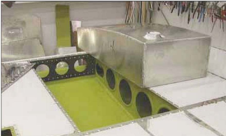
Installing the 11 gallon aux tank involves first cutting a hole in the wing, installing the mounting straps, plumbing the tank and then fabricating the cover (not supplied with kit).
