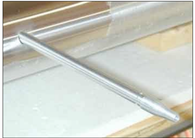
The single-mast type of pitot tube is actually one tube inside another. The inner tube receives the dynamic pressure while the space between the two tubes is vented to the outside via holes around the mast and provides static pressure. This is the view from the bottom. Bear Tracks shows how to build a single tube aluminum pitot that is similar in appearance but uses separate static ports.
