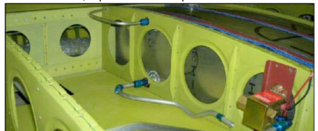
He ran the vent line from the top of the inside of the tank, around the front and out the bottom outboard.
