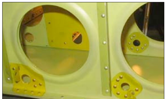
He doubled up all of his holes, which isn't necessary, although the large doubler seen on the second rib IS required, if cutting the hole bead.
