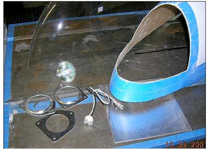
Landing lights in in the tips can be accomplished using an RV-10 lens and a light kit from Creative Air, www.creativair.com .
