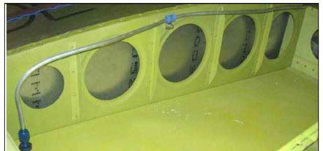
This builder vented his tanks on the "uphill" side so fuel wouldn't run out, if parked on a slope.
