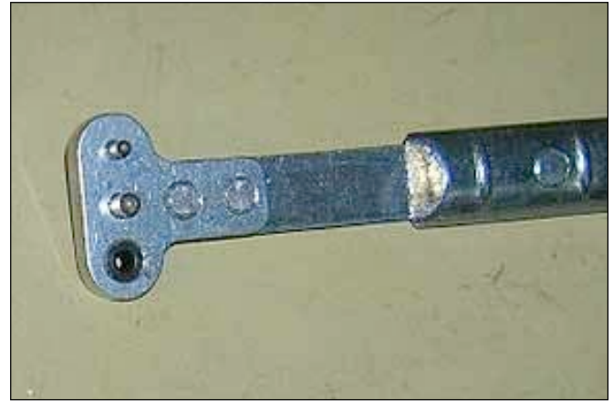
This simple little thingamabob will make drilling for your nutplates much easier. All supply houses have them.
