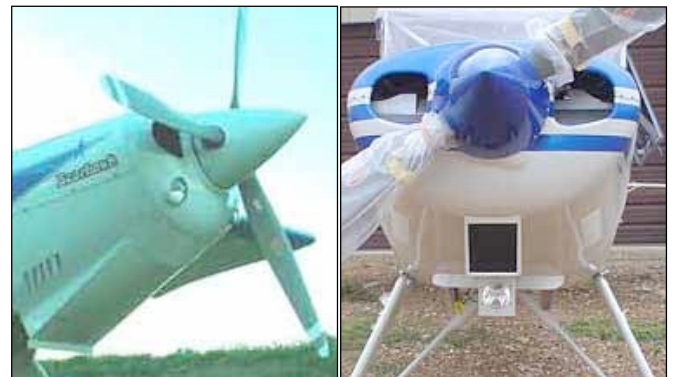
Cowl-mounted landing lights also work. The one on the right is retractable.
