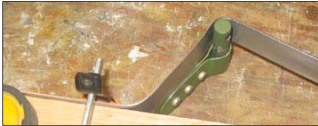
Here's a tank strap building jib used by one builder to ensure his straps were identical and to make it easier to bend them.
