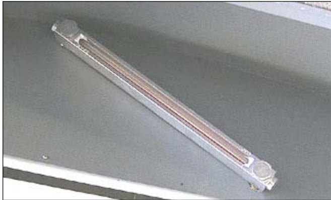
The MSC Industrial sight gauge is of industrial quality and features a cast aluminum housing. A downside is that these are GLASS and theoretically can be broken, which would empty that tank in the cockpit. A plastic cover may be called for.
