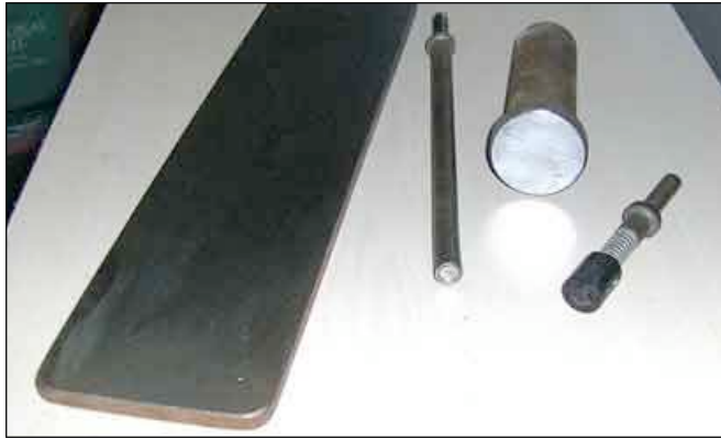
The flat plate on the left is held against the skin or laid on the bench. The rounded set at the right is a "flush bucking bar" in that it is held against the outside of the skin and the rivet set with the spring loaded nose is used on the shop end of the rivet.
